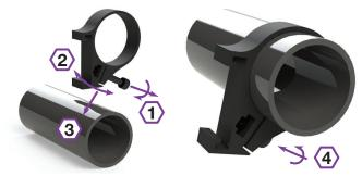
Two hardmounts are included. One for 31.8mm and one for 26.2mm round handlebars. Both can be installed in the same manner.
